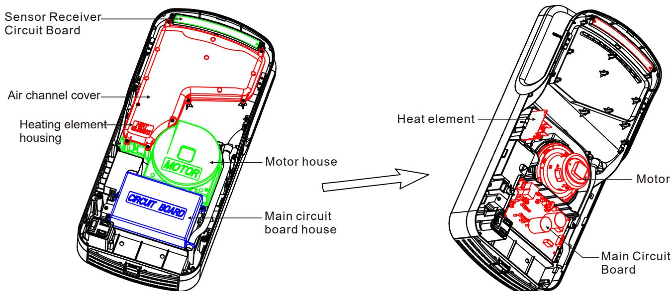
**Replace Main Circuit Board:** Move marked circuit board house cover and replace with a new right circuit board.
