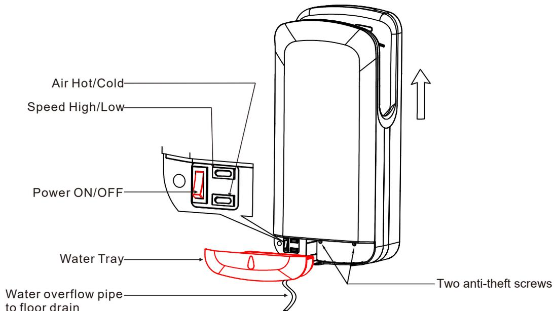
1. If the water overflow pipe is connected, please move it first.
