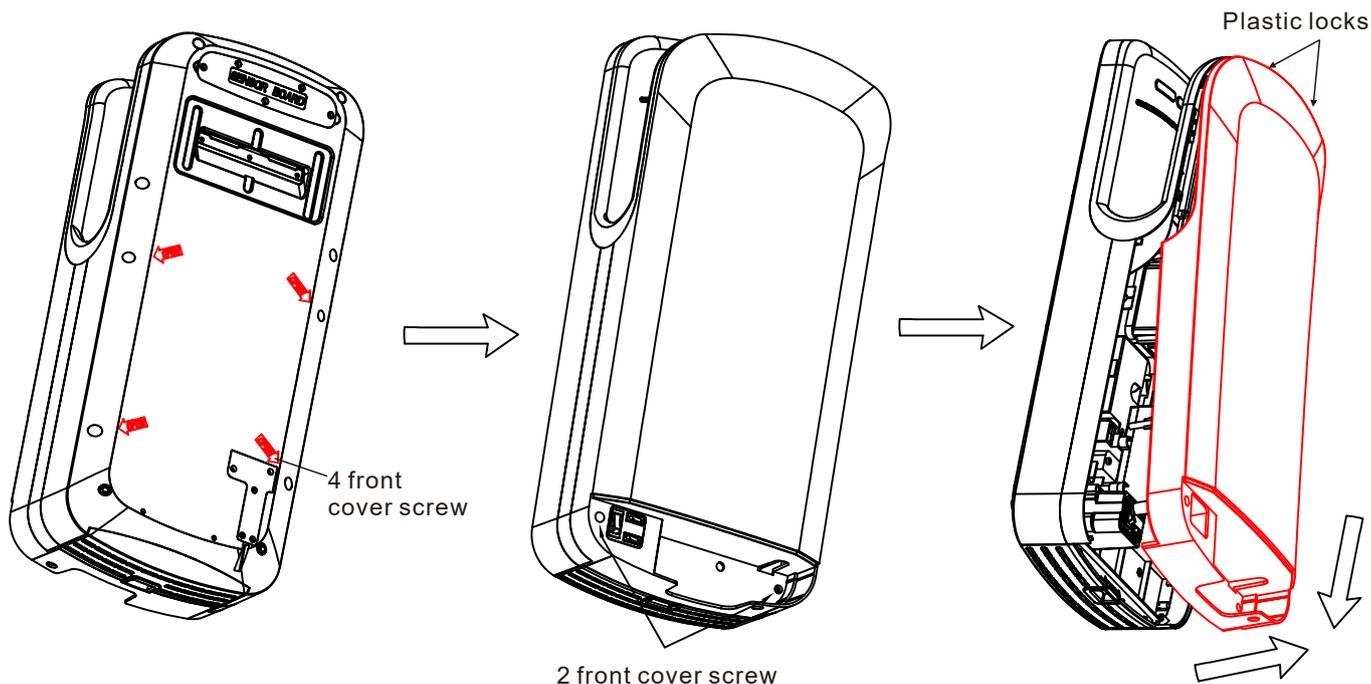
1. Remove 4 front cover screw on hand dryer back base as the arrow marked.
